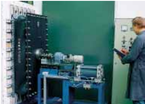
▶ Simulation test rig for expansion joints for chimney connection
