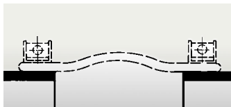
Belt connection directly on the duct
