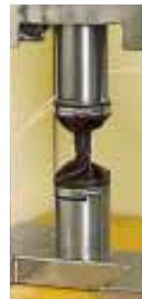
▲ Fatigue test for tensile and torsional strength
