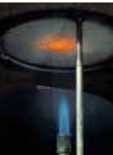
▶ Test setup for a nekal test
